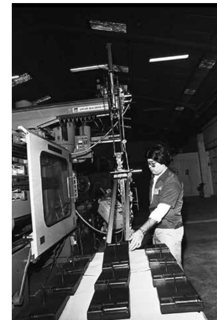
In 1981, Jeffrey Tan designed the first Singapore-made robot. Called the "manipulator", it was used in a machine which made plastic parts, such as cassette tape player covers.
